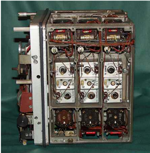
EK Receiver , top view, showing tube sockets, IF transformers and chassis compartments.
