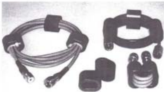
PHOTO 1: Clockwise from left: low-band ferrite choke, air-wound choke, high-band choke, the ferrite cores.
